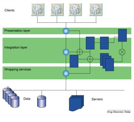
Figure 3. Heterogeneous and distributed environment. The clients at the top of the hierarchy access the data and information via a metadata rich 'integration layer'. Access to the underlying data structures and computer and application servers is mediated through the 'wrapping services', which maintains the information necessary to bind and direct the queries to the correct source.
